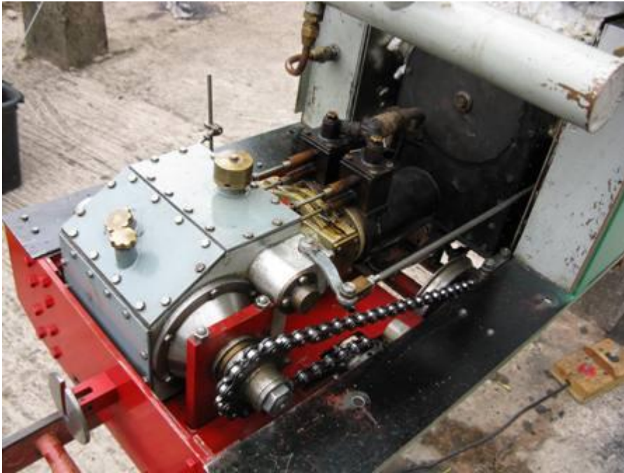
A sneaky look under Jess' bonnet showing the very efficient uniflow steam wagon engine and the front of the locomotive type boiler: a winning combination that always performs well. On this occasion Jess returned an efficiency of 1.709%, not the best ever but a nice reflection on Mike's driving skills and Ron's engineering.
